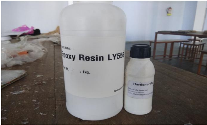
Figure 2: Epoxy (LY 556) and hardener (HY951)
